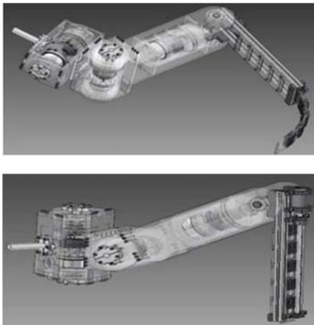
Fig. 3. Walking leg design (bottom) and swimming leg design (top) modes of the bio inspired robot [5].
